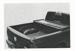
3. Please square the Tonneau cover up to the side bed rails and front bed wall so it is even on all three sides.
